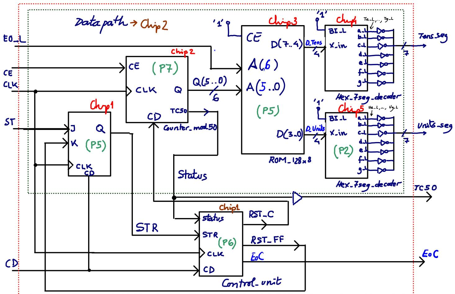
status signal is '1' when  $CE=1$  and  $Q$  is at last state
