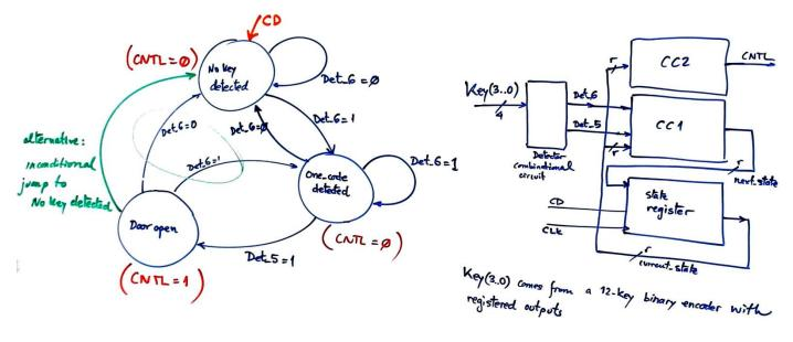
A standard <u>P8</u> dedicated processors including a datapath for solving comparison applications. The secret code is *information* easily saved and modified using switches. In the datapath two chained 4-bit data registers save the last two *Key* sampled values, and a comparator with "65" generates a status signal to control state transitions. This system is easy upgradable to 4-digit or longer secret key. This is an example project <u>D2.8</u>.
