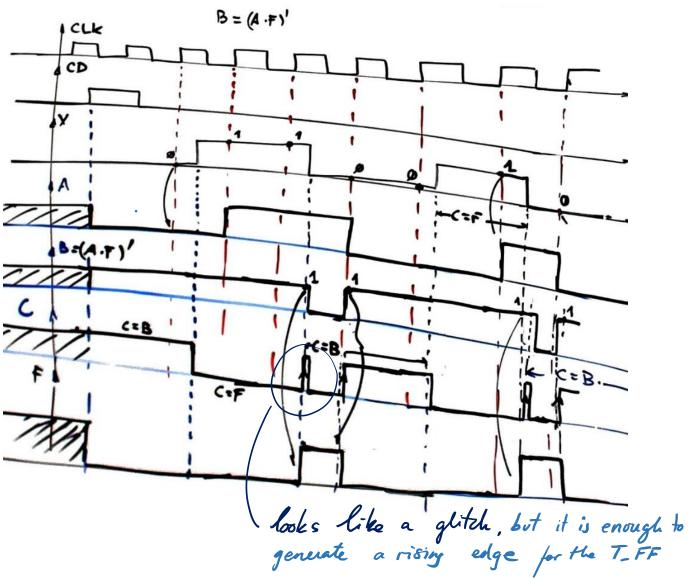
F pulse width depends on the delay between & falling odge and CLLE rising edge
