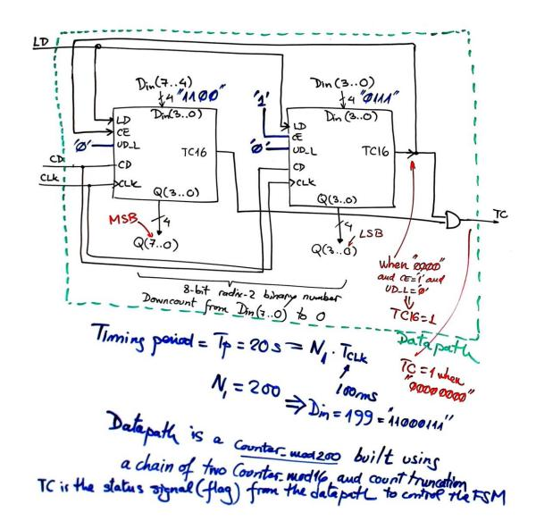
Counter is loading in parallel continuously when Idle and down counting when timing
