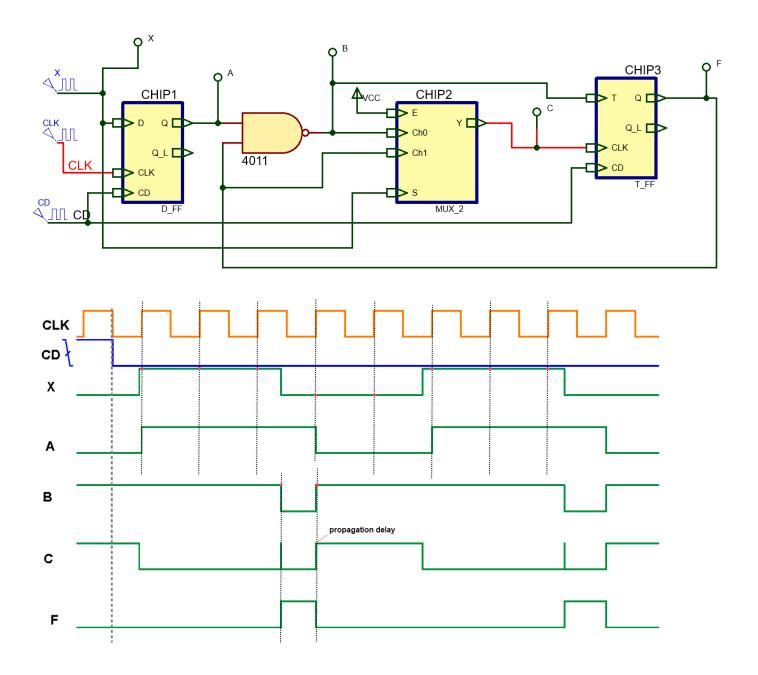
This is the timing diagram from Quartus Prime project and ModelSim targeting a MAXII CPLD device (project files available in DIGSYS).
