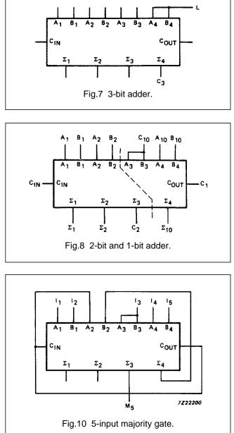
inputs are equally weighted. The outputs  $\sum_{0}$ ,  $\sum_{1}$  and  $\sum_{2}$  produce a binary number equal to the number inputs (I<sub>1</sub> to I<sub>5</sub>) that are HIGH. Figure 10 shows a method of implementing a 5-input majority gate. When three or more inputs (I<sub>1</sub> to I<sub>5</sub>) are HIGH, the output M<sub>5</sub> is HIGH.
