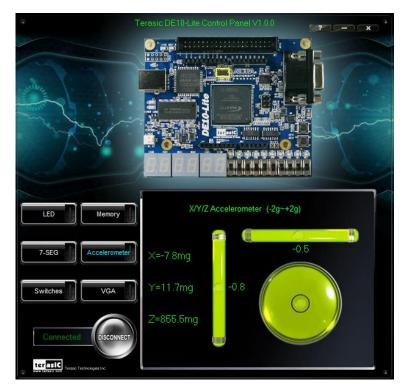
Figure 2-7 Level by G-Sensor
