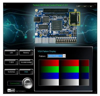
Figure 2-8 Controlling VGA display under Control Panel
