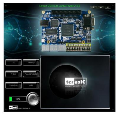
Figure 2-1 The DE10-Lite Control Panel
