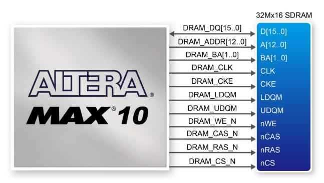
Figure 3-23 Connections between the SDRAM and MAX 10 FPGA
