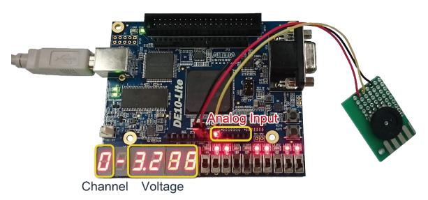
Figure 5-11 7-Segment display the measured channel and voltage
