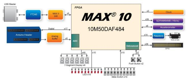
Figure 1-4 Board Block Diagram
