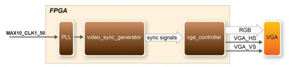
Figure 5-5 Block diagram of the VGA Pattern demonstration
