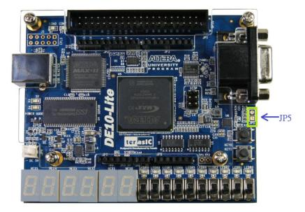
Figure 6-1 JP5 position on the DE10-Lite board.
