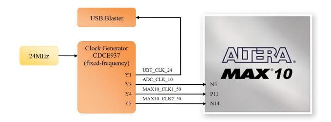
Figure 3-12 Clock circuit of the FPGA Board
