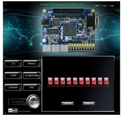
Figure 2-3 Controlling LEDs
