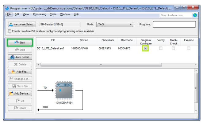
Figure 3-9 Program .sof file into the FPGA device
