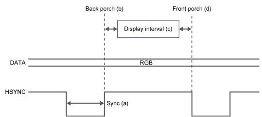
Figure 3-22 VGA horizontal timing specification
