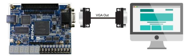
Figure 5-7 The setup for the VGA Pattern demonstration
