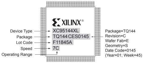
Part marking for non-chip scale package
