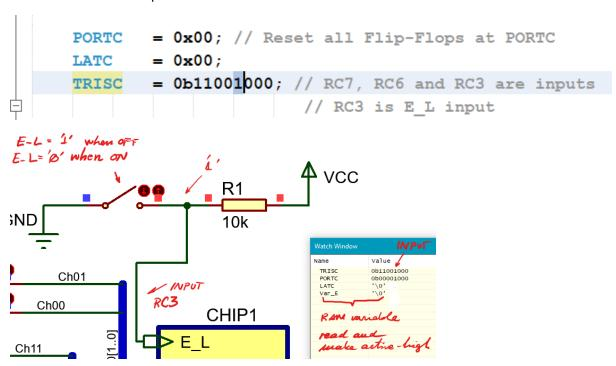
Let us simulate an error when configuring TRISC3: there is the switch as input circuit but TRISC3 is ='0' (meaning that it is output!!) . The switch cannot be polled and reading DO NOT work.
