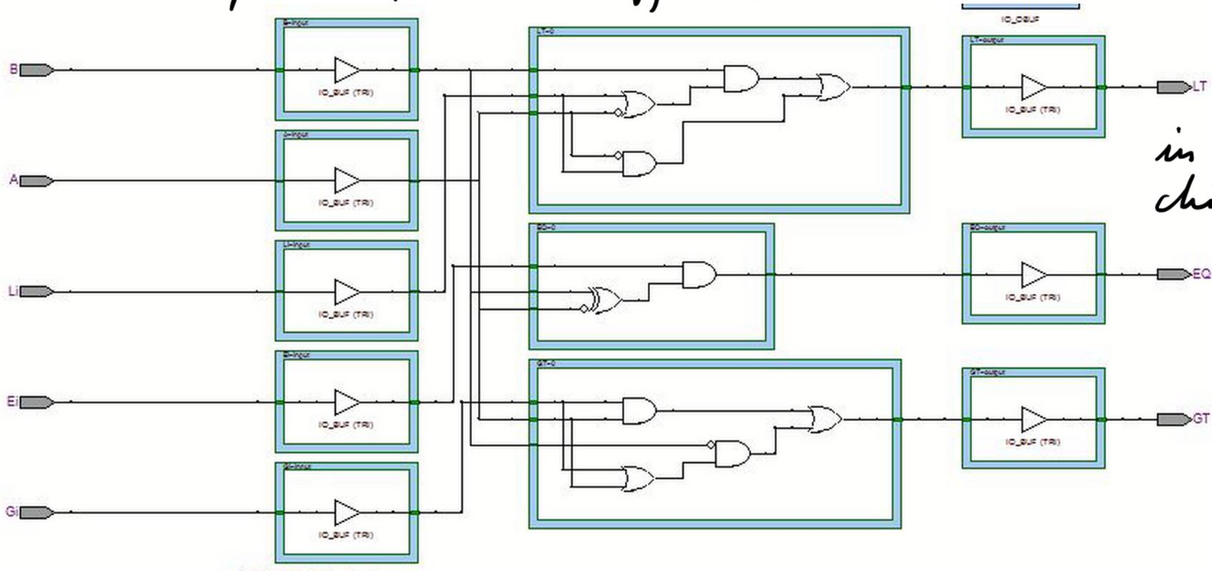
logic implemented in the target chip Cyclone III
