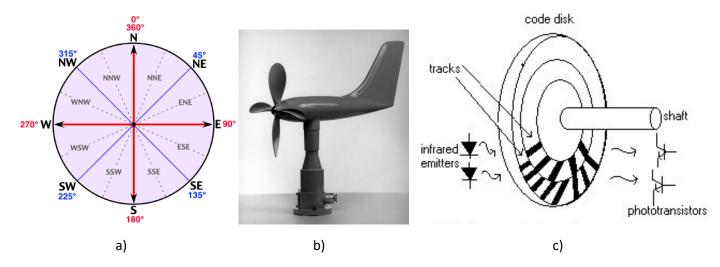
Fig. 1 a) Wind compass describing the sixteen principal bearings used to measure wind direction, b) the wind <u>transducer</u>, and c) the basics of the Gray to binary rotary <u>encoder</u> sensor.
