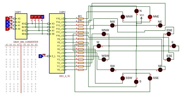
Fig. 2 Electrical schematic. The picture is showing Gray code "1001", which is "1110" in binary and corresponds to the wind direction Nord-Nord-Est "NNE".
