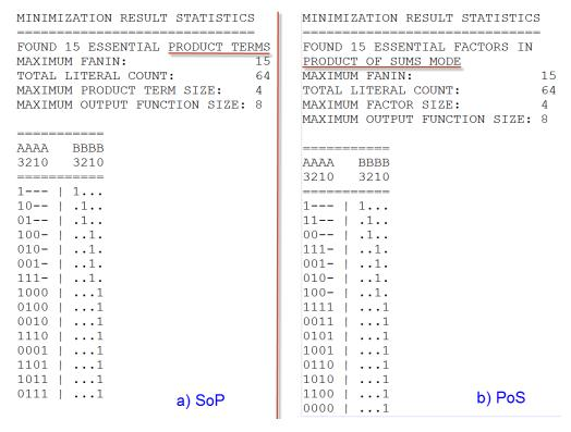
Fig. 3 Table output from MInilog when minimising the Gray\_Bin\_Converter Chip1. a) Sum of products (SoP), b) PoS.
