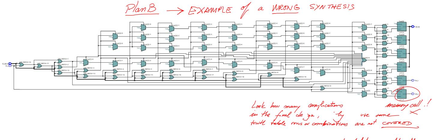
Memory cells such latches or flyp-flop registers MUST NOT be here
