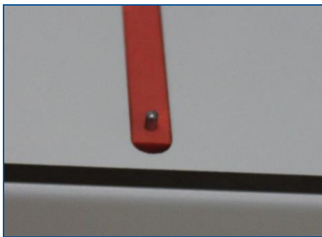
Fig. 56: Inserted dowel pin
