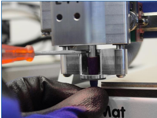
Fig. 19: Loosening the locking screw
