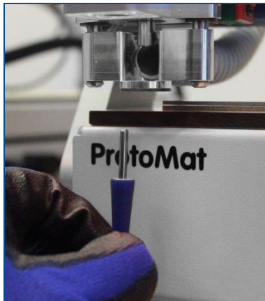
Fig. 20: Extracting the dummy tool
