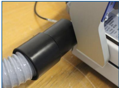
Fig. 12: Connecting the extraction system
