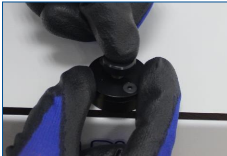
Fig. 55: Inserting the dowel pin
