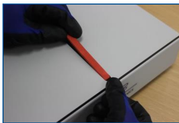
Fig. 48: Inserting the reference-hole strip
