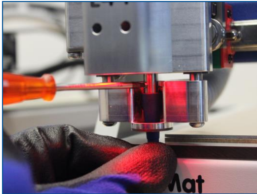
Fig. 62: Loosening the locking screw
