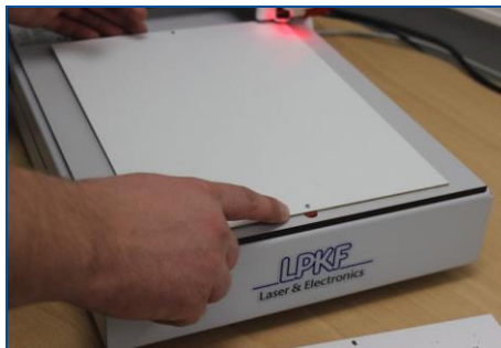
Fig. 35: Processing table with drilling underlay plate
